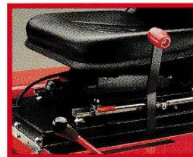
Deluxe suspension seat with variable load setting adjusts easily to the operator's height.
