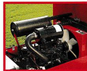
Kubota 3-cylinder, liquid-cooled diesel engine for better power and fuel economy.
