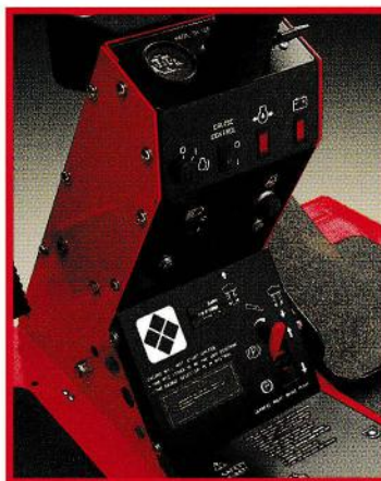
Instrument panel includes oil pressure, water temperature, and alternator warning lights. Hourmeter, throttle, parking brake light and light switch are on the instrument panel for operator convenience.
